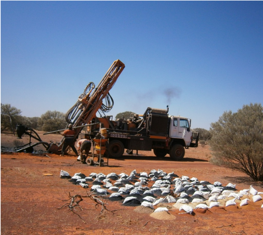
Figure 2 – RAB drilling in progress at Mooloogool. See sulphidic black shale samples in foreground.
